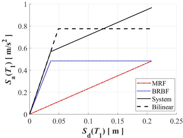
Figure 2: Design components and system capacity curves.
