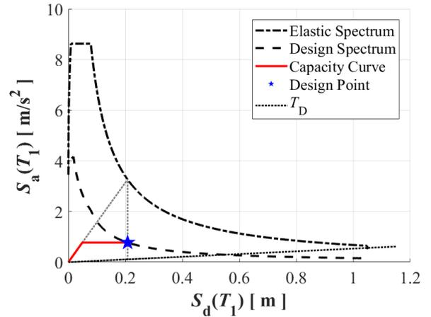
Figure 3: Performance point of the equivalent SDOF.
