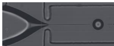
Figure 2.10: Tip streaming in a flow-focusing geometry (Anna, 2016).
