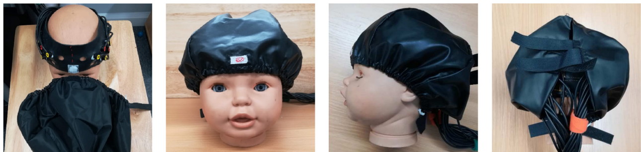
Figure 8. Headcap used to shield fNIRS headband from near infrared light. The cap is attached to the fNIRS headgear at the infant's forehead using Velcro. The lower edge of the headband has elastic spanning the lower rim of the fNIRS cap. Velcro strips in the back of the headband allow quick adjustment for different head sizes to prevent delays in capping.
