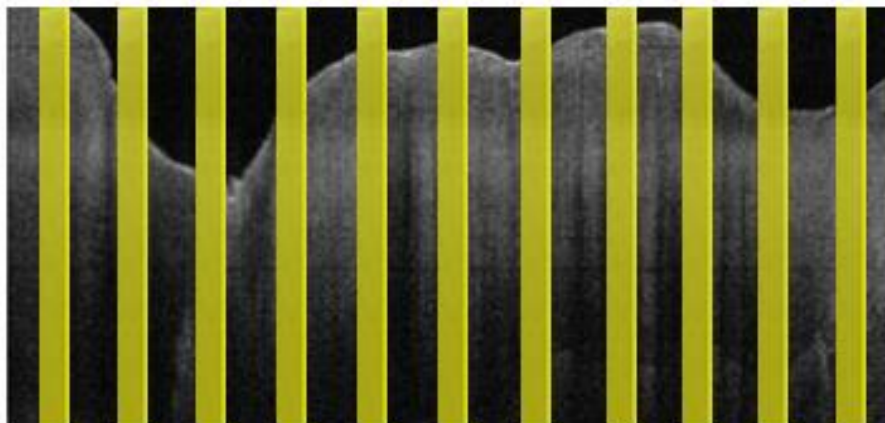
Figure 8.1: Demonstrating schematic description of the distribution of the regions chosen throughout a B-scan of sample 13 ICDAS score 1, with the yellow boxes resembling a 10-pixel width of scan
