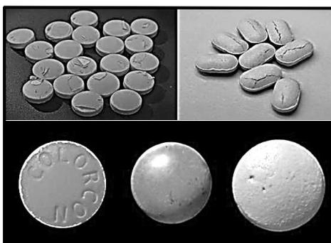
Figure 1.3: Tablet defects. Pictures taken from Muliadi and Sojka (2010).
