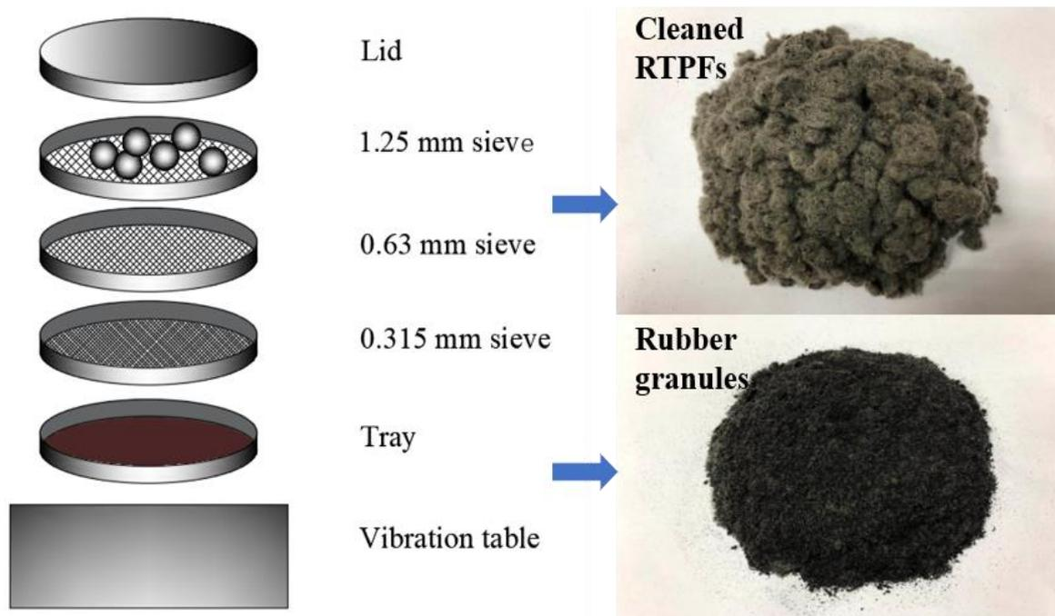
**Fig. 3.** A schematic diagram showing the process of estimating the composition of RTPF
