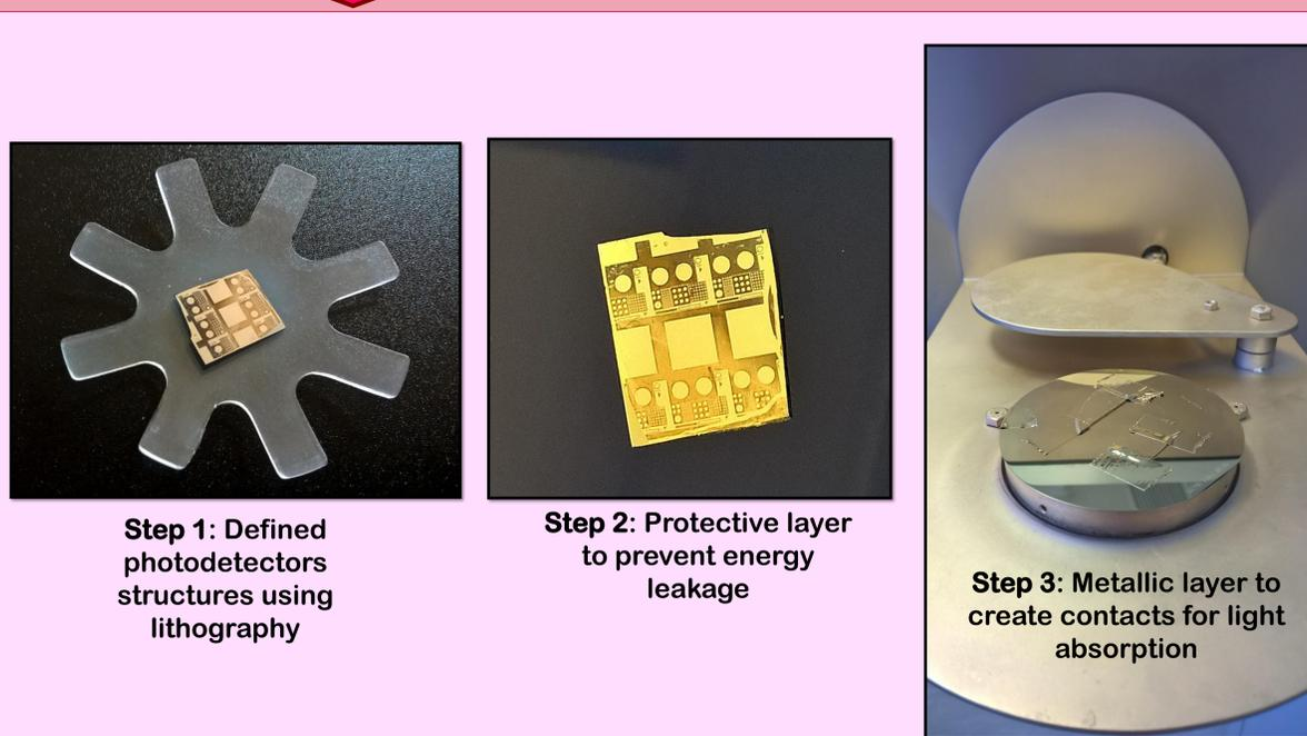
Figure 2: Fabrication Step by Step
