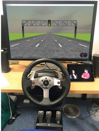
Figure 1: Driving simulator setup with steering wheel, pedals, monitor, and iPad for secondary task.
