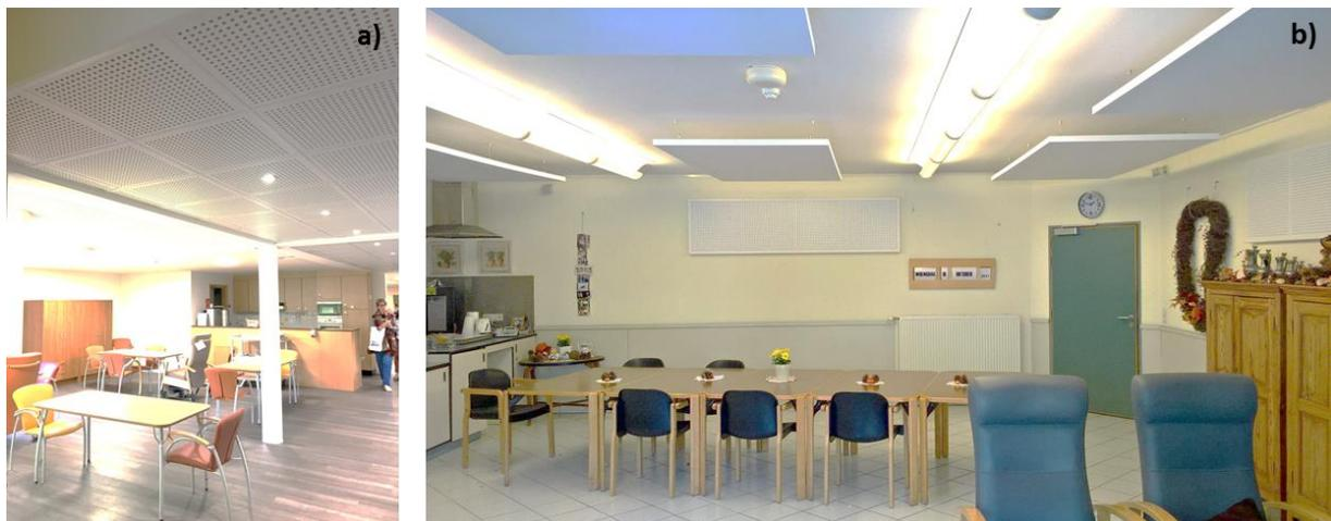
**Figure 6 – Overview of the acoustic interventions in the living rooms: a) dining room with absorbing ceiling panels (Gyproc) and acoustic floating floor in VH; b) living room with absorbing ceiling panels (DOX-Acoustics) and wall panels (Gyproc) in LH.**
