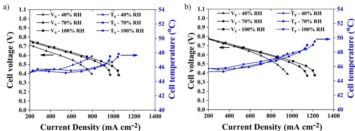
Fig. 6: Cell temperature during polarisation curve measurements for (a) single-serpentine flow-field and (b) lung-inspired flow-field at 40% RH, 70% RH and 100% RH. (Legend:  $V_S$  – cell voltage with serpentine flow-field;  $V_F$  – cell voltage with fractal flow-field;  $T_S$  – serpentine flow-field temperature;  $T_F$  – fractal flow-field temperature).
