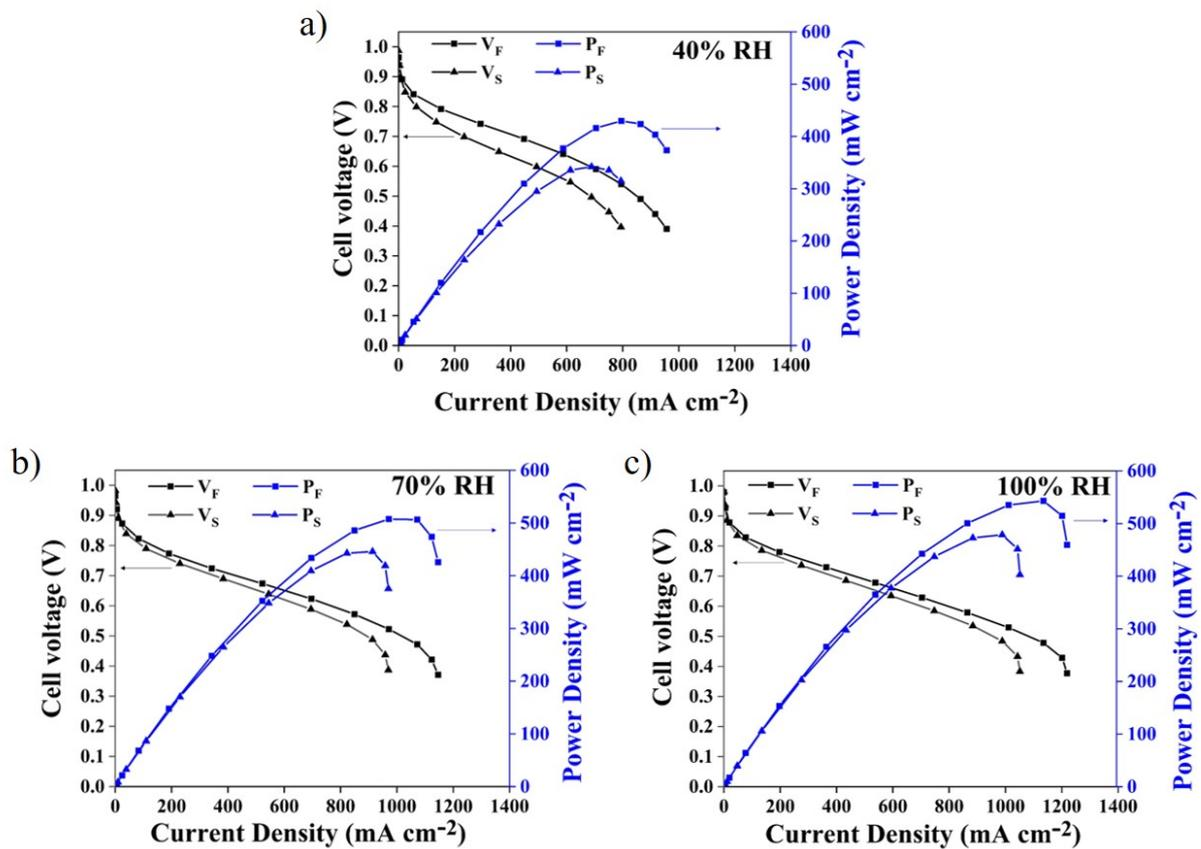
Fig. 5: Polarisation curves at (a) 40% RH, (b) 70% RH and (c) 100% RH. (Legend: V<sub>F</sub> – cell voltage with fractal flow-field; V<sub>S</sub> – cell voltage with serpentine flow-field; P<sub>F</sub> – power density with fractal flow-field; V<sub>S</sub> – power density with serpentine flow-field).
