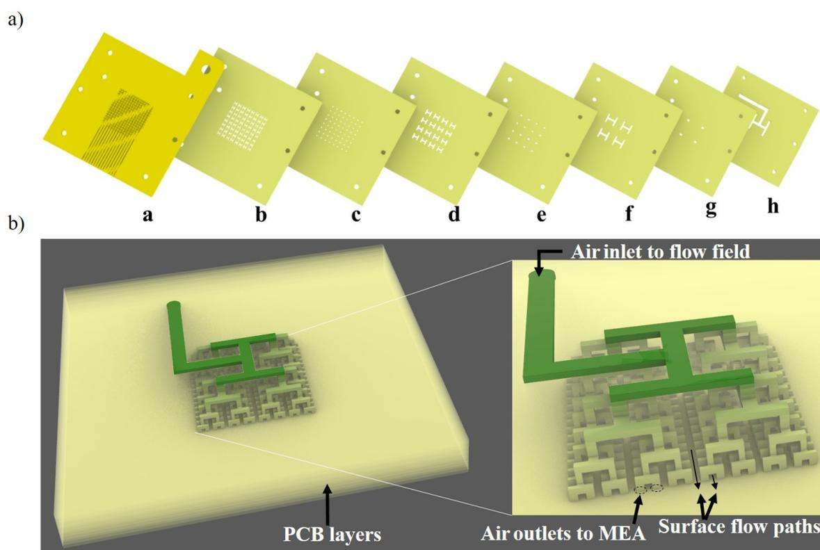
Fig. 1: (a) PCB plates a-h comprising 2D planar individual layers of hierarchical fractal flow-field geometry. (b) RHINO model depicting the assembly of individual PCB layers, resulting in a fractal flow-field geometry. Shown are the single air inlet, multiple air outlets to MEA level, and the surface flow paths for the cathode air and water outlets from the fuel cell.
