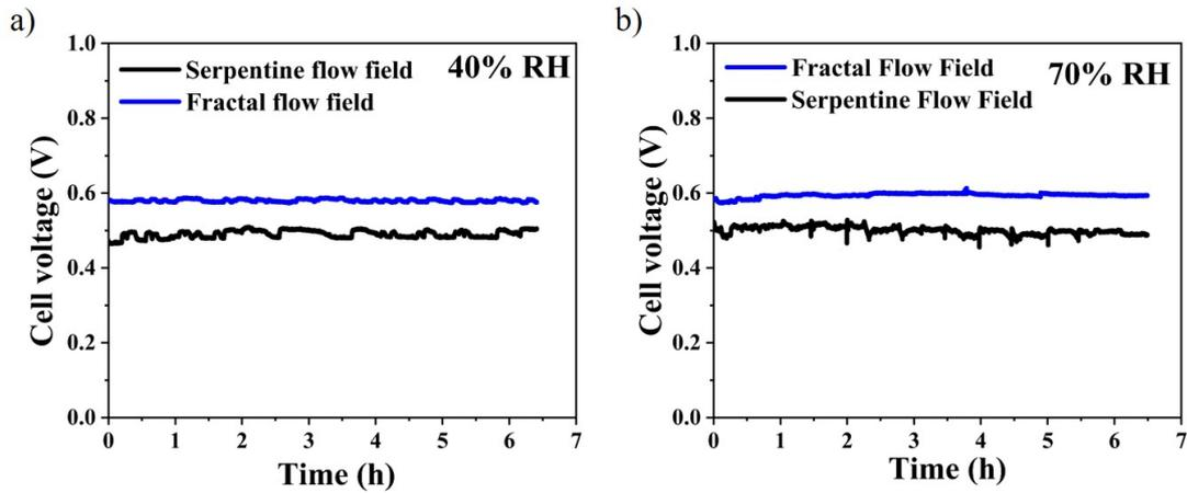
Fig. 8: Cell voltage fluctuation over 6 h during galvanostatic tests at (a) 40% RH and 700 mA cm<sup>-2</sup> and (b) 70% RH and 750 mA cm<sup>-2</sup>.
