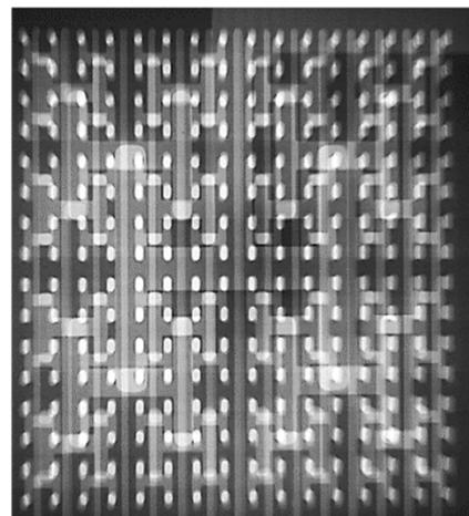
Fig. 3: (a) Experimental setup for X-ray CT scanning, (b) radiograph of the region of interest (ROI) of the scanned lung-inspired flow-field.
