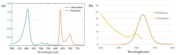
Figure 2: The excitation and emission spectra of PpIX (a) and CdTe quantum dots (b).
