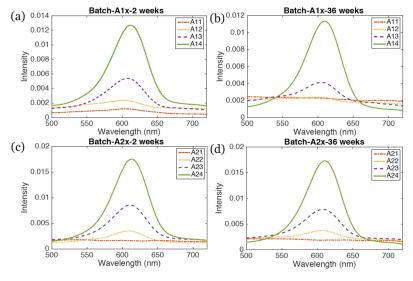
Figure 5. Optical absorption and reduced scattering spectra of the phantom batches with varying titanium dioxide and quantum dots concentrations. Optical absorption,  $\mu_a$ ; Optical reduced scattering,  $\mu_s$
