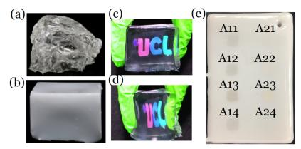
Figure 1. (a) Native gel wax, (b) Native gel wax with TiO2 and Carbon Black ink as additives, (c, d) Squashing a gel wax phantom with inclusions having complex geometry (e) The composite phantom. (a-d) are adopted from Ref [10] with permission.
