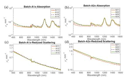
Figure 4. Optical absorption and reduced scattering spectra of the phantom batches with varying titanium dioxide and quantum dots concentrations. Optical absorption,  $\mu_a$ ; Optical reduced scattering,  $\mu_s$
