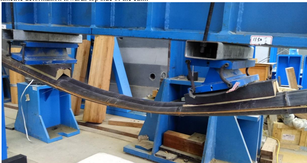
Figure 5. Typical failure of bamboo poles during bending test
