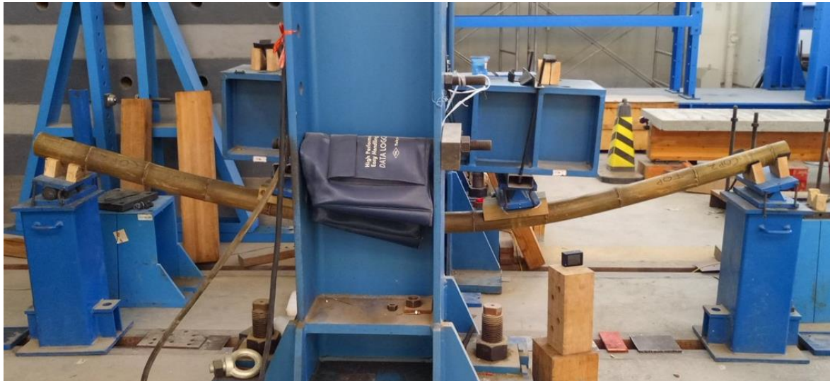
Figure 4. Asymmetric deformation towards top side of the culm
