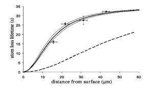
FIG. 6. Data: lifetimes for the loss of atoms trapped above the videotape atom chip with a 400-nm gold layer. Solid lines: the theory of Scheel *et al.* at temperature  $350\pm50$  K. Dashed line: expected lifetime near a 4- $\mu$ m-thick gold layer.
