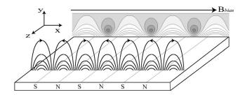
FIG. 1. Magnetic field lines produced by the magnetized videotape are shown in the foreground. A uniform bias field,  $B_{bias}$ , is added to this to make an array of atom guides. Contours of constant magnetic field strength are shown in the background. Circular contours enclose the lines of minimum field strength, where atoms are trapped.
