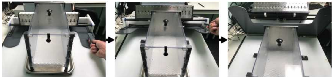
Figure 5-2 The modified BATA apparatus showing the platform and handle which enables the inversion of the entire rig prior to presentation to the rats.
