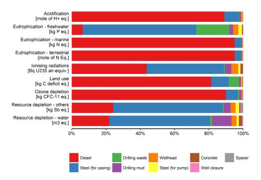
Figure S4 - Detailed hot-spot analysis on the construction and the end of life of the production well for the impact categories not included in the main paper.
