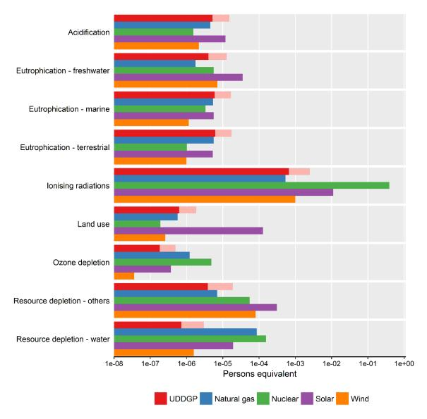
Figure S5 - Comparison of the normalised environmental impacts of 1 kWh of electricity produced from UDDGP with natural gas in combined cycle gas turbines, nuclear pressurised water reactors, utility-scale solar photovoltaic and offshore win farms.
