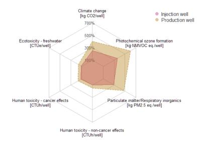
Figure S6 - Radar chart comparing the environmental impact scores in six environmental impact categories due to wells construction and decommissioning in the UDDGP project (injection and production wells) and the Hellisheidi geothermal plant in Iceland.
