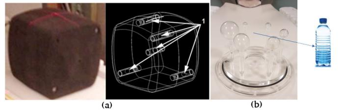
**Fig. 1:** (a) VQC Phantom with five small  $^{68}\text{Ge}$  spheres and (b) Bladder Mimicking Bottle Phantom which consists of 6 fillable spheres and a 500 ml bottle placed between smallest spheres.
