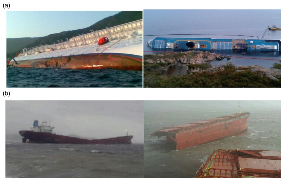
Figure 2. Typical example of grounding damaged vessels. (a) Costa Concordia (a cruise ship), which was grounded in front of Italy Sea (Pedersen 2015). (b) Pacific Carrier (a bulk carrier), which was grounded in South Korea Sea (ChosunBiz 2012) (Left = first grounded condition, Right = break into two parts by a typhoon). (This figure is available in colour online.)
