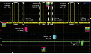
Fig. 6. Oscilloscope traces of: (top) downlink and SPI signals (SCK, MOSI, MISO) with acknowledgement response from a PI through SPI link; and (bottom) 3 PIs establishing SPI communication when addressed with respective ID codes.
