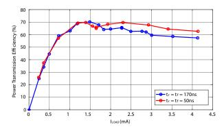
Fig. 7. Power transmission efficiency (PTE) of the power delivery to varying of load current. (Red) rise and fall time of power carrier square wave tr =tf= 50 ns; (blue) tr =tf= 170ns.
