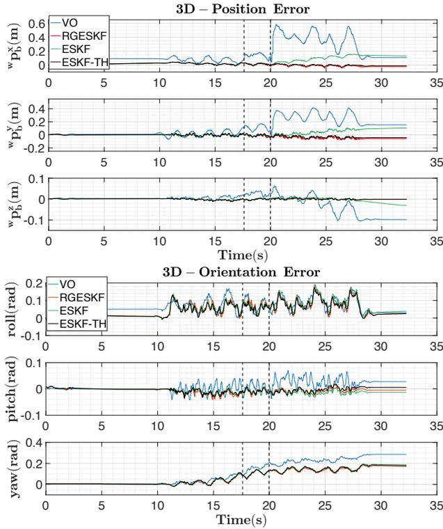
Fig. 3. **Top**: 3D - position error, **Bottom**: 3D - orientation error for the WALKMAN 2.0 - VO experiment, blue lines indicate the VO, red lines the proposed Robust Gaussian ESKF, green lines the ESKF, and black lines the finely tuned ESKF-TH. The first vertical dotted line corresponds to when a human enters the FoV of the camera, while the second one when he removes a strong feature source for VO which diverges.
