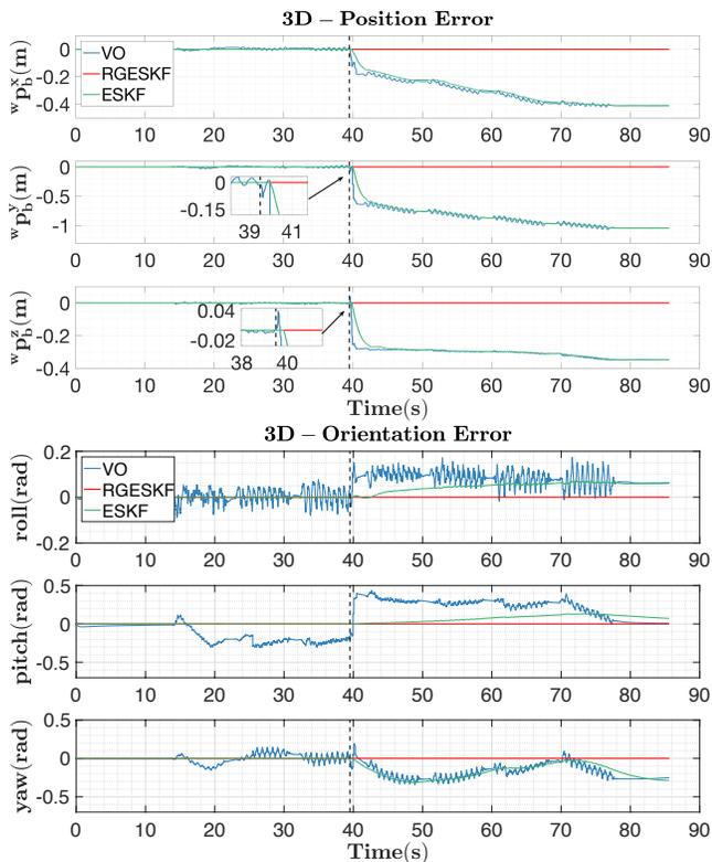
Fig. 4. **Top:** 3D - position error, **Bottom:** 3D - orientation error for the NAO - VO experiment, blue lines indicate the VO, red lines the proposed Robust Gaussian ESKF, and green lines the ESKF. The vertical dotted line specifies when a human removes a strong feature source for VO which diverges.
