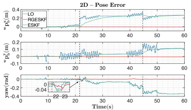
Fig. 5. 2D - pose error, for the NAO - LO experiment, blue lines indicate the LO, red lines the proposed Robust Gaussian ESKF, and green lines the ESKF. The vertical dotted lines corresponds to when a human suddenly covers the robot's LiDAR with a box, causing LO to diverge.
