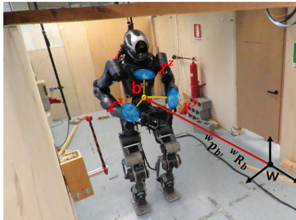
Fig. 1. Illustration of frames used in base estimation on the 29DoF WALK-MAN v2.0 humanoid robot:  $w$  corresponds to the inertial world frame,  $b$  is the base frame, and blue ellipses indicate the orientation uncertainty.
