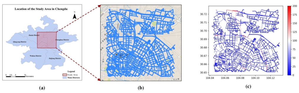
Figure 6. Location of study area and the road network. (a) Location of study area. (b) Road network of study area. (c) Concrete example of generated traffic flow.
