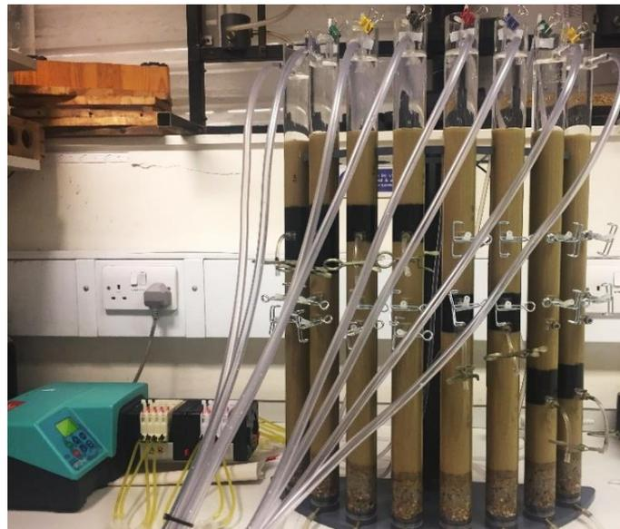
**Figure 3.8 The GAC sandwich biofilter system setup.**
