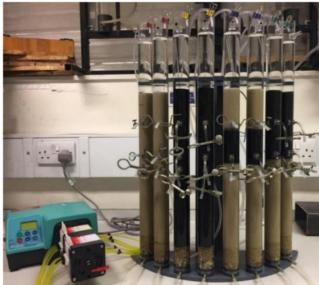
**Figure 3.6 Schematic of biofilter column set-up.** Sand, GAC, GAC sandwich, and anthracite-sand dual biofilters were set-up in duplicate (from left to right).
