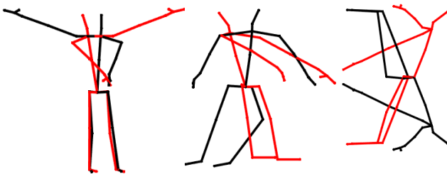
Fig. 5. Skeleton reflection in the x-direction (Left), y-direction (Middle), z-direction (Right): original skeleton in black, reflection in red.
