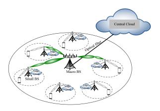
Fig. 1. An illustration of two-tier HetNets equipped with edge clouds associated with the SBSs and central cloud connected by the MBS via optical fiber, where the MBS provides central cloud computing services for UEs through restricted MIMO/massive MIMO backhaul for addressing more complicated computing tasks which cannot be handled by the SBSs' edge cloud due to the limited computing capability.
