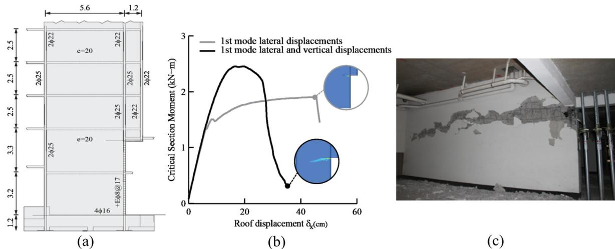
Figure 4. Building analysed: (a) elevation of a resisting plane of building in Santiago (dimensions in meters); (b) pushover results for the moment-displacement curve with (black line) and without (grey line) vertical deformations; and (c) observed damage pattern reproduced analytically.
