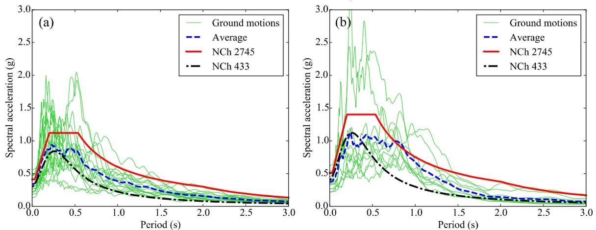
Figure 5. Design spectra from the NCh433 and NCh2745 Chilean seismic codes, and from recorded ground motion accelerograms of the 2010 Chile earthquake near to the fault plane (from 33°S to 38.5°S), in soil type II, and: (a) zone II (central valley), and (b) zone III (coast).
