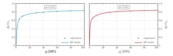
Figure 4: Plastic increment in the void ratio  $\Delta e^p$  as a function of the forming pressure  $p_c$ . Experimental data (dots) are compared with the Cooper and Eaton model, eq. (2.3), (solid line) for two water contents: w = 5.5% (left) and w = 7.5% (right). Note that there is a  $\approx 8\%$  (hardly visible) difference between the experimental values reported in the two graphs, due to the different water content.
