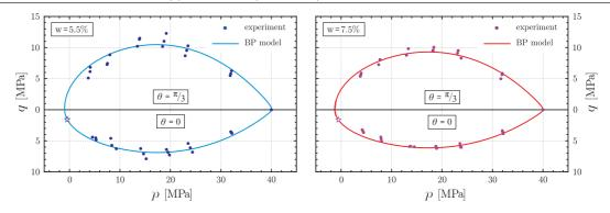
Figure 9: Meridian sections of the yield locus at Lode's angles  $\theta = \pi/3$  and  $\theta = 0$  for aluminum silicate green body formed under uniaxial strain at  $p_c^* = \sigma_1 = 40$  MPa, with water contents of 5.5% (left) and 7.5% (right). Yield points from triaxial tests (dots), evaluated through linear regression, and from equi-biaxial flexure tests (stars) are fitted with the BP yield surface (Bigoni and Piccolroaz, 2004), corresponding to the material parameters listed in Table 3.
