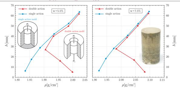
Figure 5: Mean (across the transversal area) density  $\rho$  distribution along the sample height h for water contents w = 5.5% (left) and 7.5% (right). For each water content, the double pressure forming technique with a final pressure  $\sigma_1 = 40$  MPa is compared to the that obtained with the single action device. Note that the distributions of density are significatively more uniform in the former case than in the latter.
