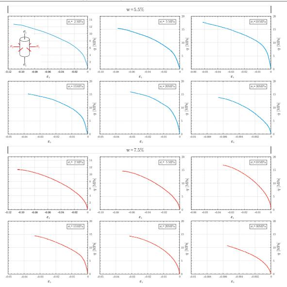
Figure 8: Triaxial extension tests at different axial stress  $\sigma_1 = \{2, 5, 10, 15, 20, 30\}$  MPa (from left to right) on samples with w = 5.5% (upper part) and w = 7.5% (lower part) of water content. Each curve represents the average of values from three different tests with the same set-up (water content and axial stress). The tests have been terminated before failure.
