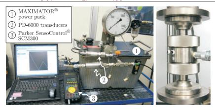
Figure 6: The experimental set-up for the high-pressure triaxial loading tests. Note the equipment to measure the lateral pressure (on the left) and the 45-D0554 Hoek cell inserted in the ZwickRoell Z250 electromechanical testing machine (on the right).
