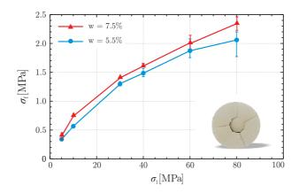
Figure 11: Flexure strength  $\sigma_f$  vs. forming pressure  $\sigma_1$  evaluated from equi-biaxial flexure tests performed on ceramic tablets with water content 5.5% (circle) and 7.5% (triangle). The post-mortem sample is shown in the inset.
