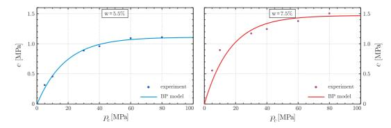
Figure 12: Cohesion parameter c as a function of the forming pressure  $p_c$ . Experimental data relative to aluminum silicate powder are compared to the model of increase of cohesion, eq. (4.6), proposed by Piccolroaz et al. (2006a) (solid line), evaluated with the parameters of Table 4, for water contents 5.5% (left) and 7.5% (right).
