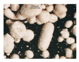
Figure 1: I14730 aluminum silicate spray dried powder in the loose state: bulk material (left) and micrograph at 31.5x (right, obtained with a Nikon stereoscopic microscope Nikon SMZ-800 equipped with Nikon Plan Apo 0.5x objective and a Nikon DS-Fi1 high-definition color camera head). The granules have an irregular surface and a mean diameter of  $425 \mu m$ .
