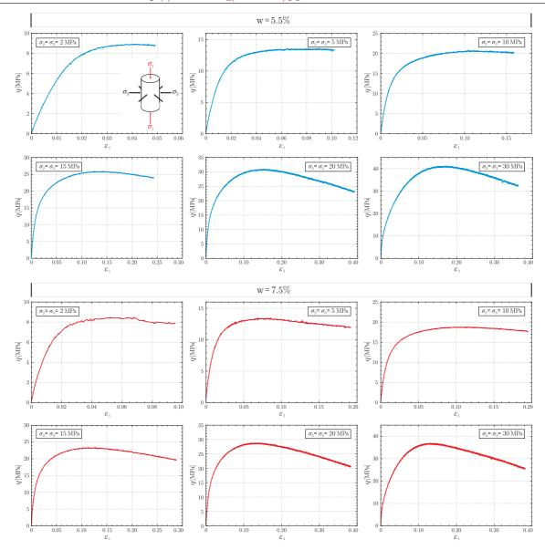
Figure 7: Triaxial compression tests at different cell pressures  $\sigma_2 = \sigma_3 = \{2, 5, 10, 15, 20, 30\}$  MPa (from left to right) on samples with w = 5.5% (upper part) and w = 7.5% (lower part) of water content. Each curve represents the average of values from three different tests with the same set-up (water content and lateral pressure).
