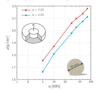
Figure 3: Logarithmic plot of density  $\rho$  vs. forming pressure  $\sigma_1$  obtained through uniaxial strain tests (see the inset on the left) on samples (shown in the inset on the right) with water contents w = 5.5% (circle) and w = 7.5% (triangle). Each curve corresponds to an average value taken over five tests, deviation was found to be negligible.
