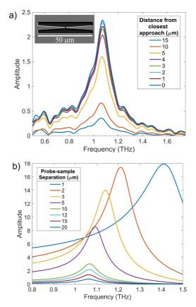
**Fig 1**. a) Experimentally measured Fourier transform spectra of a single resonator for varying probe-sample separation; the inset shows an SEM image of resonator. b) Simulated Fourier transform spectra of a single resonator for varying probe-sample separation.
