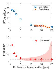
**Fig 2** a) Peak simulated FT amplitude with experimental peak FT amplitude fitted b) Simulated peak FT frequency (with spectral curve overlay for comparison to linewidth).
