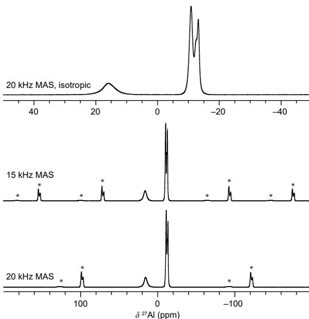
Figure S8:  $^{27}\text{Al}$  solid-state NMR spectra of  $\text{Al}_2(\text{MoO}_4)_3$  at different MAS speeds. Spinning sidebands move with MAS speed and are denoted with asterisks. Spectra were recorded at 16.4 T.
