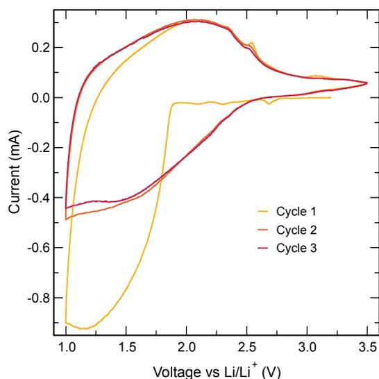
Figure S2: Cyclic voltammogram of  $\text{Al}_2(\text{MoO}_4)_3$  with 3 cycles against Li metal in a two electrode Swagelok cell. The first cycle differs substantially from the following cycles.
