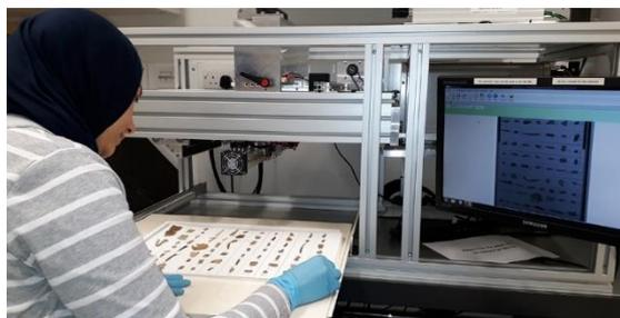
**Figure 5-1.** Hyperspectral Imaging Scanner
