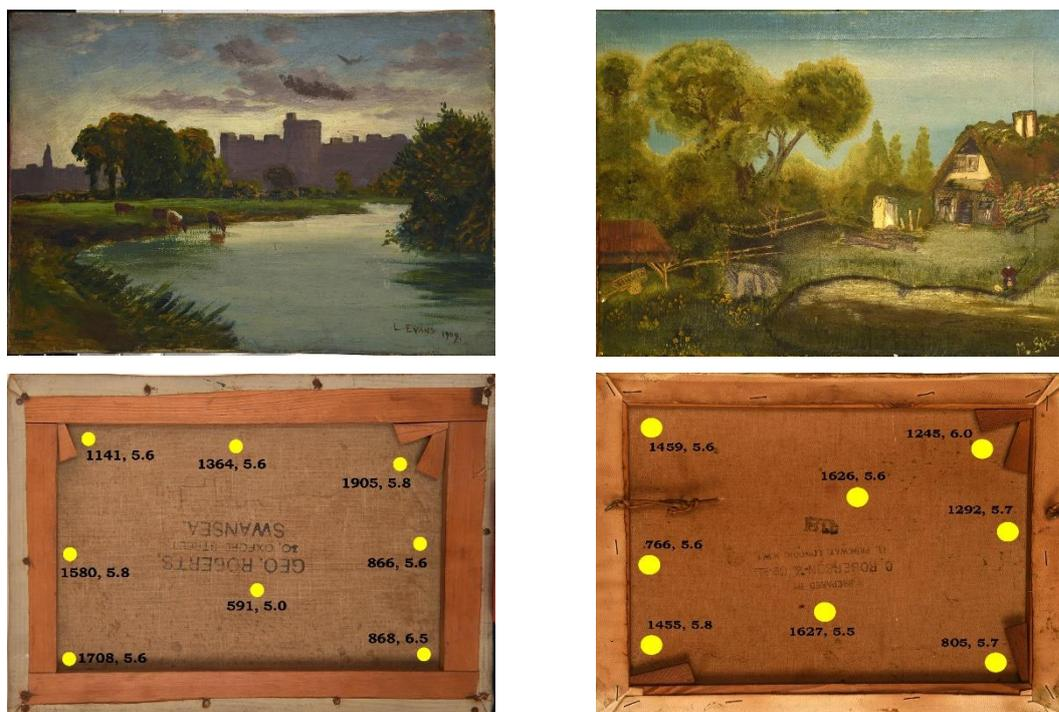
**Figure 5-6.** The results of the pH and DP predictions for two painting canvases; P8 (left, bottom) and P9 (right, bottom) from the UCL-ISH collection based on the developed regression calibration models. Yellow dots representing the different selected positions for the spectral measurements. The top row shows the front side of the two paintings; P8 (left, top) and P9 (right, top).
