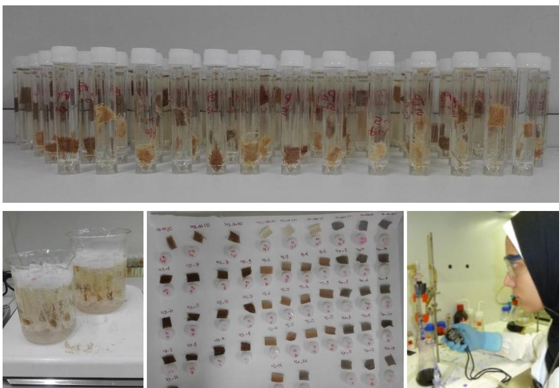
**Figure 2-9.** DP measurement experiment of canvas samples, showing the special preparation process needed for the samples due to the heavy glue and paints.
