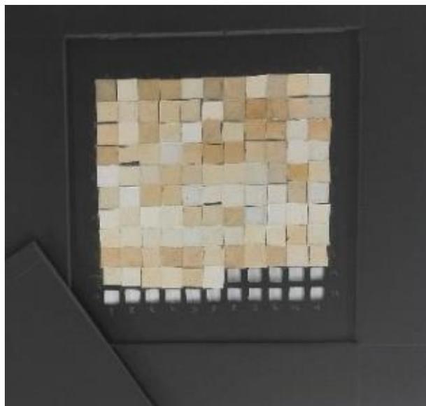
**Figure 2-3.** Calibration target with 105 characterized samples of Islamic paper (Front and back sides).
