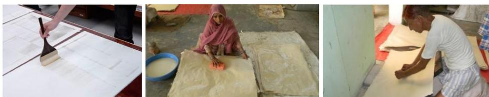
**Figure 2-1.** Application of sizing (left and middle) and polishing (right) techniques on paper. © (left) [http://precious-piece.com/?page\\_id=2358](http://precious-piece.com/?page_id=2358), © (right and middle) <http://www.hussainpapers.co.in/gallery.htm>.
