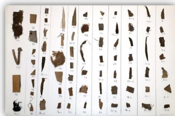
**Figure 2-6.** Calibration target with 72 well-characterized samples of painting canvases (16<sup>th</sup> – 20<sup>th</sup> C.).
