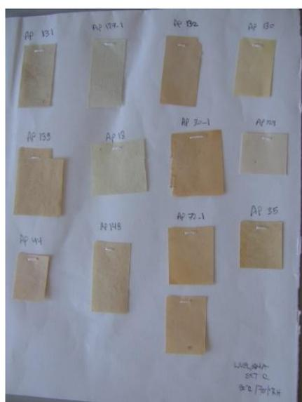
**Figure 2-10.** Some of the Islamic paper and canvases samples during one of the accelerated degradation experiments.
