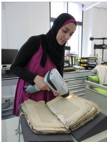
**Figure 4-12.** Collection of spectral data using PHAZIR handheld NIR instrument (Polychromix) in the interval 1600 – 2400 nm from the Wellcome Library Islamic collection.
