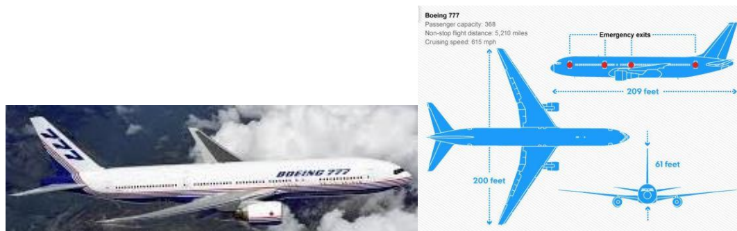
Figure 10. Principal dimensions of a Boeing 777 airplane.
