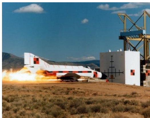
Figure 6. The impact test between a F4 Phantom and a concrete wall (Sugano et al. 1993).
