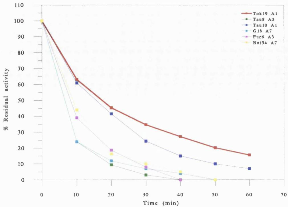
Figure 3.10 Thermostability profiles of the crude esterase preparations at 80°C
