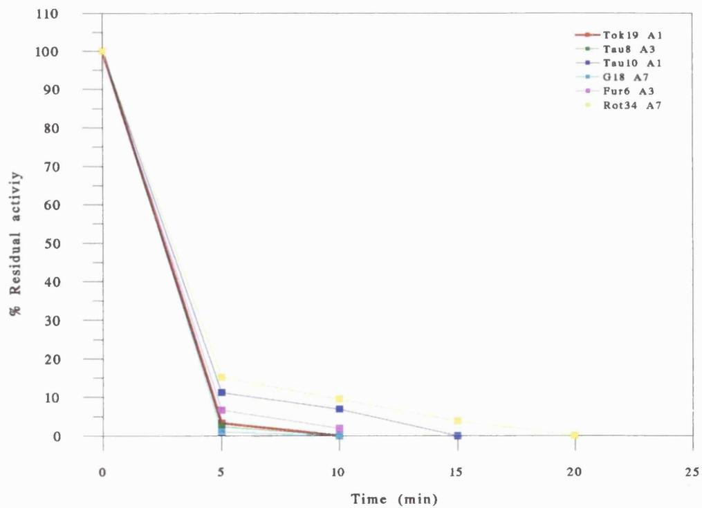
**Figure 3.11 First order thermostability log<sub>e</sub> plots for the crude esterase preparations at 75°C**
