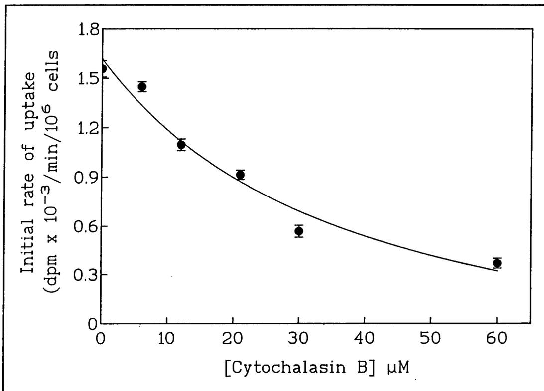
Fig. 3.7. Effect of cytochalasin B on 2-deoxy-D-glucose transport. Transport assay was carried out essentially as described in Section 2.6. The ability of cytochalasin B to inhibit the uptake of 2dGlc was determined as described in the legend to Fig.3.6. The curve represents the best fit of the data to equation 3.2. Each data point is the mean of triplicate estimations.
