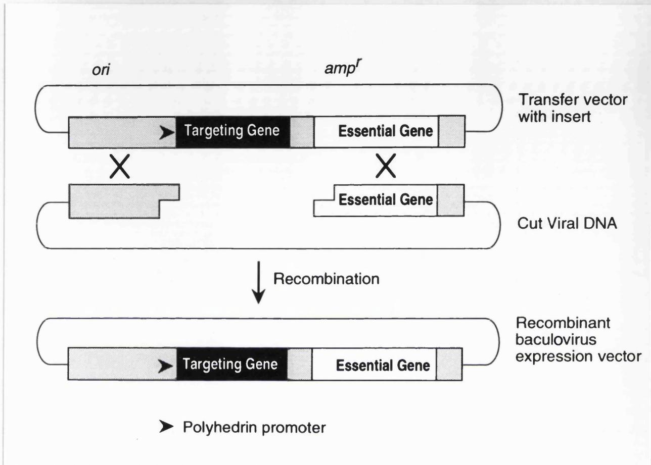
Fig. 6.3. Illustration of allelic replacement reaction between recombinant transfer vector and viral DNA containing the lethal deletion.
