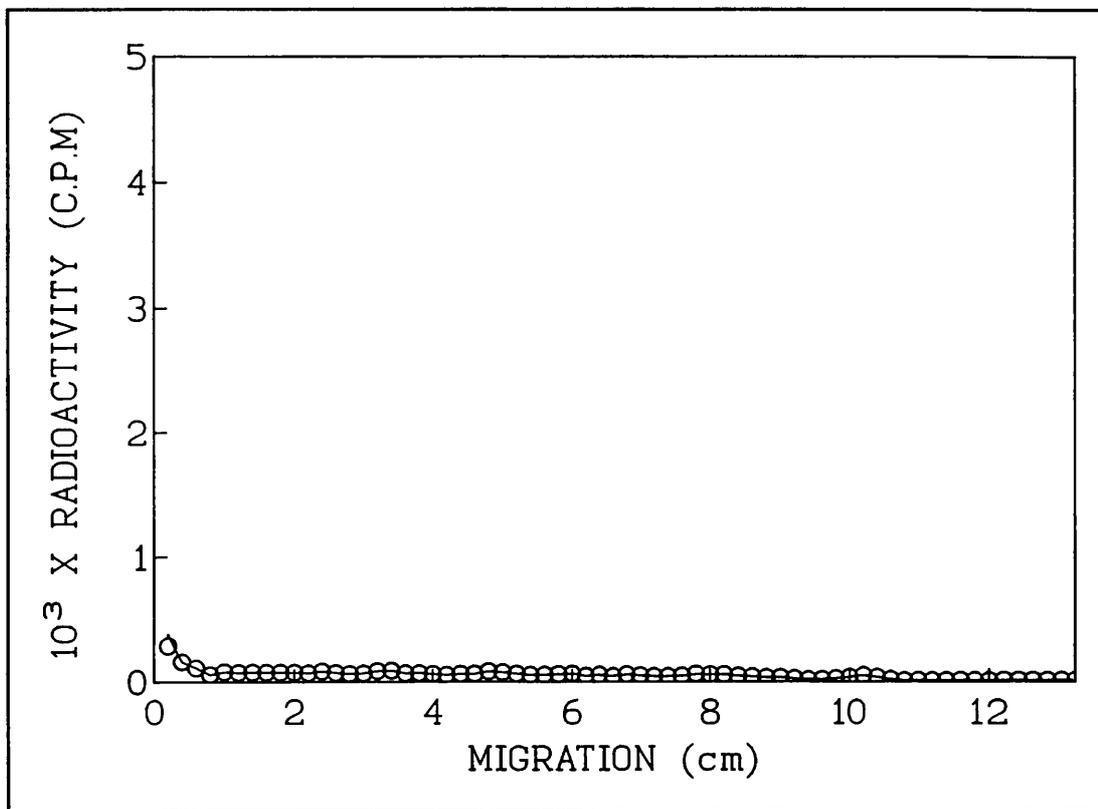
Fig. 5.20. Electrophoretic profile of photoaffinity labelling of uninfected insect cells. Non-infected Sf9 cell membranes were photoaffinity-labelled with [<sup>3</sup>H]cytochalasin B in the presence of 500 mM-L-glucose, as described in the legend to Fig. 5.19.
