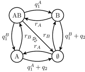
**FIGURE 4.** Continuous time Markov chain for a 2 component system with common cause failure. Arrows denote possible transitions, and arrow labels denote transition rates. The node *AB* represents a fully working system, *A* a system where only *A* works, *B* a system where only *B* works, and  $\emptyset$  a system where neither component works.
