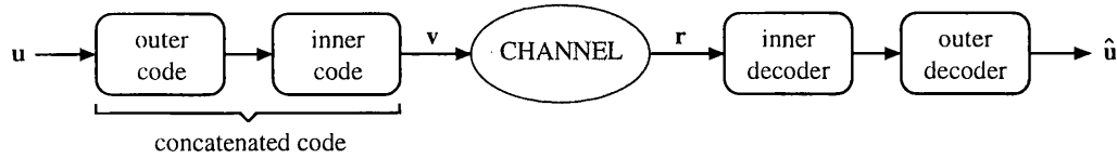
Figure 2.3 Block diagram of a concatenated coding system.
