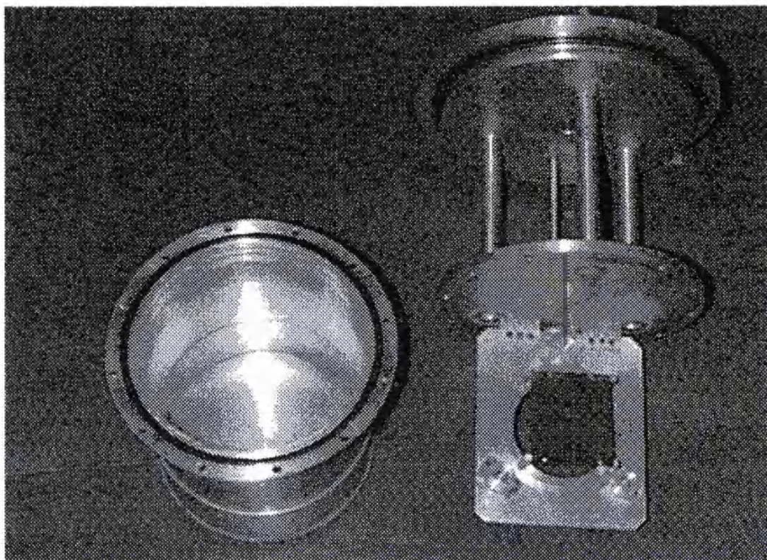
Figure 5.1a. Picture of the sample container showing the vanadium plates and the cylindrical can in which they were sealed.
