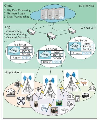
FIGURE 1. The system architecture of fog-computing-based radio access networks.
