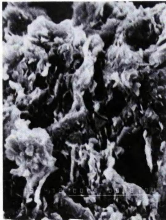
Plate 4.3.6 SEM photographs for the most weathered sample, Taiwan. (c), (d): random orientation and pore enlargement can be observed.
