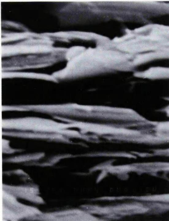
Plate 4.3.4 SEM photographs for the least weathered sample, Taiwan. (a), (b): preferred orientation of the clay particles along scaly surface.
