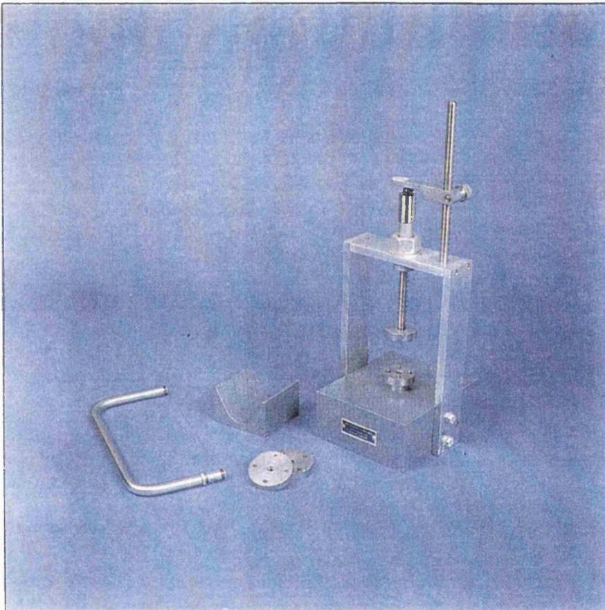
Figure 5.2.4 Manual soil lathe and trimming saw used to produce cylindrical specimen for triaxial testing
