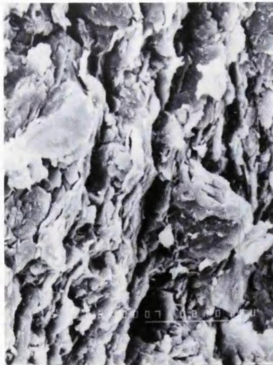
Plate 4.3.5 SEM photographs for the partially weathered sample, Taiwan. (a), (b): remnant preferred orientation of the clay particles.
