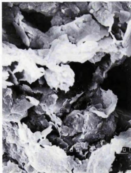
Plate 4.3.6 SEM photographs for the most weathered sample, Taiwan. (a), (b): no preferred orientation of the clay particles exist.
