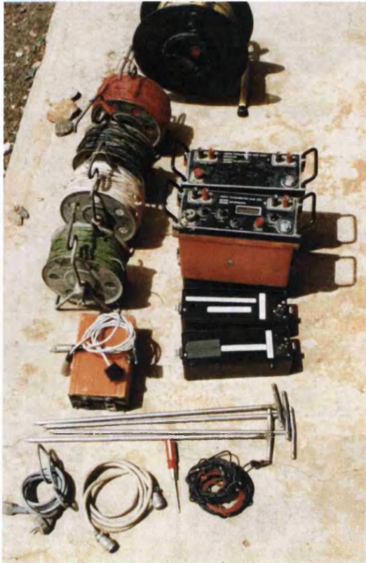
Figure 3.19 ABEM Terrameter and cables used for resistivity surveys.
