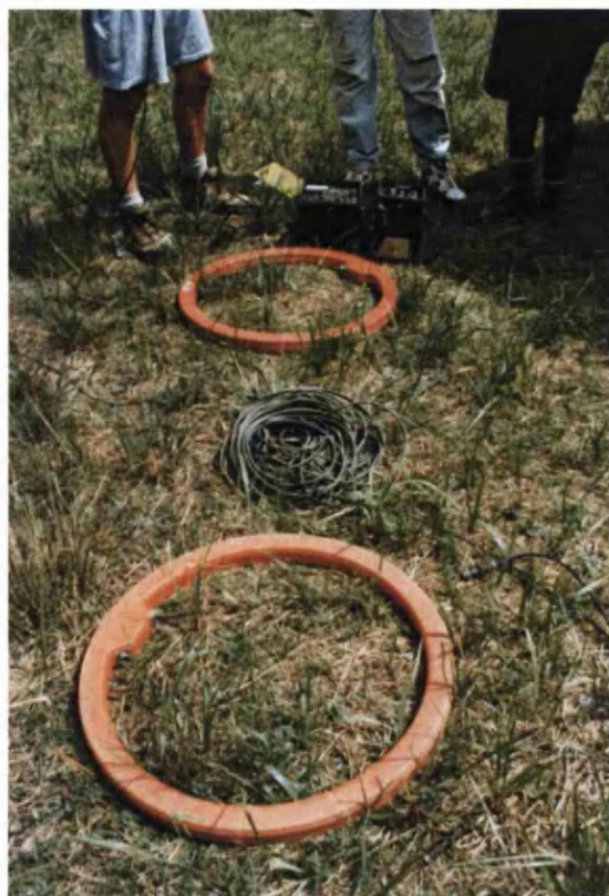
Figure 3.17 Geonics EM34 equipment, comprising two coils, a connecting cable, transmitter and receiver.
