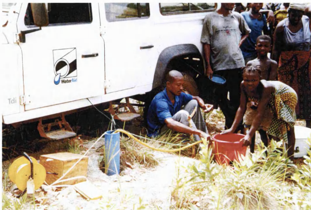
Figure 3.21 A pumping test using whale pumps at Ochingini village.
