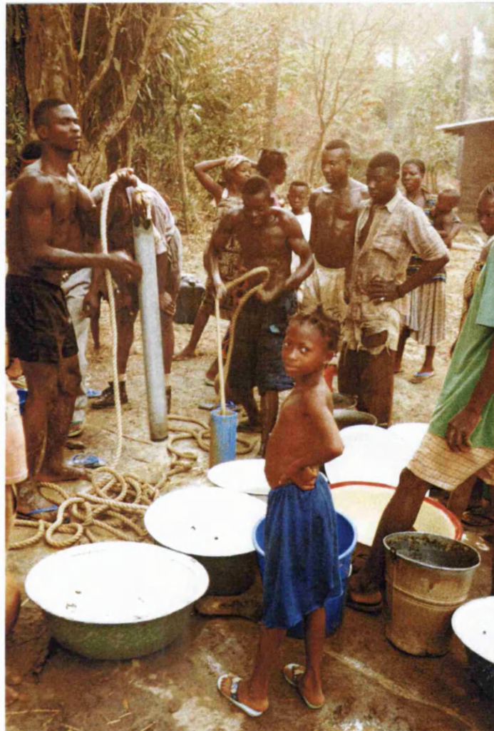
Figure 6.12 Community members carrying out a bailer test at Edumoga village, Oju.
