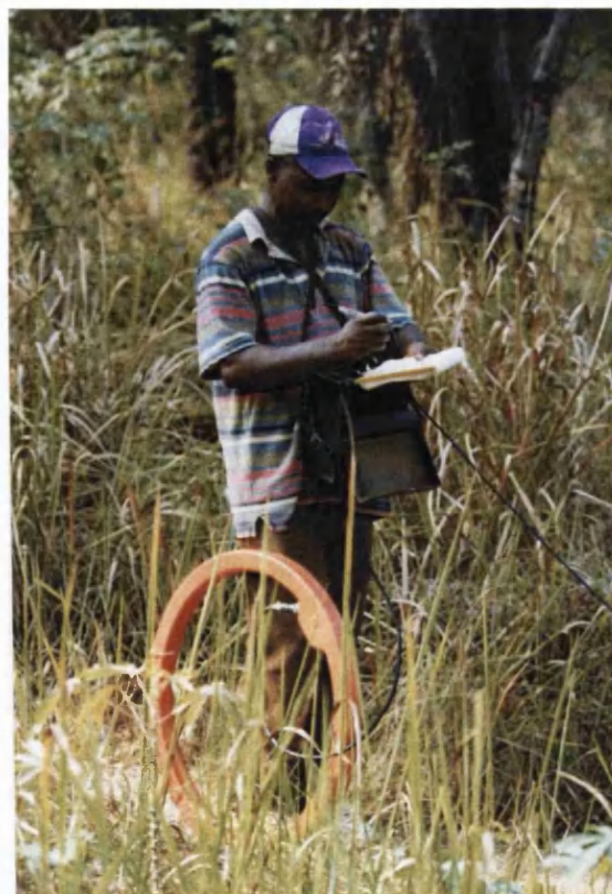
Figure 3.18. The Geonics EM34 equipment used with horizontal dipoles.
