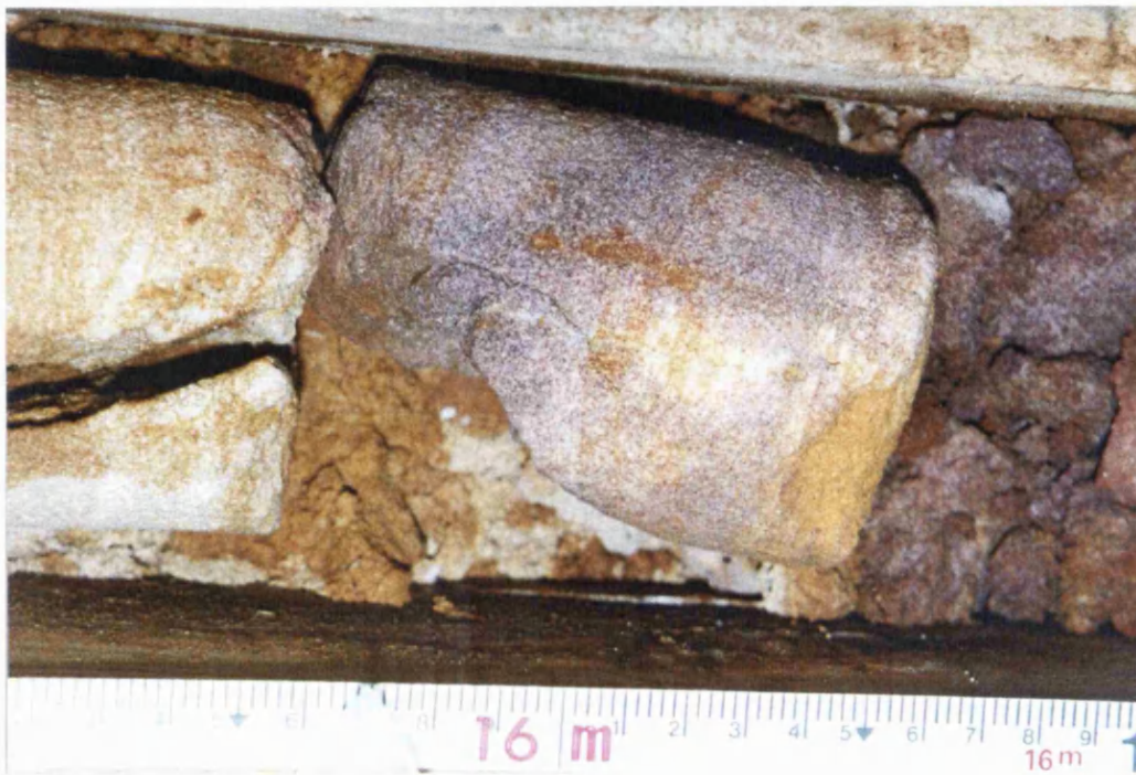
Figure 5.6 Photograph showing sub vertical fracture (far left) in a core from the Makurdi Sandstone (BGS7, 16 m).
