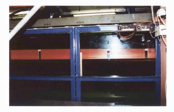
Figure 5.10 Load applied on pontoon module 4 in single array with Hinged-Rigid connection
