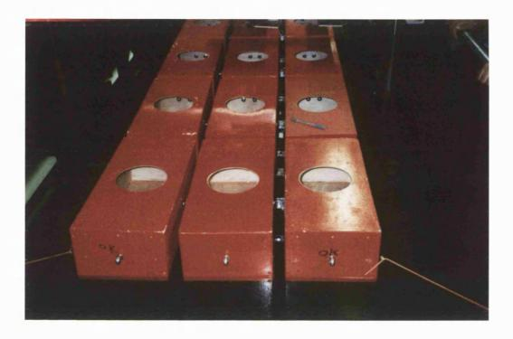
Figure 5.6 Assembly pontoons for hinged connection for mat array
