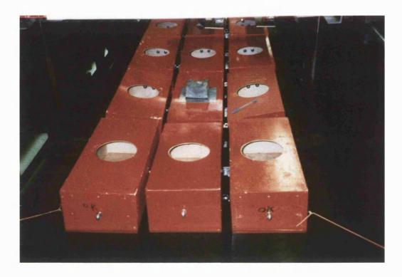
Figure 5.12 Load applied on pontoon module 2 and 4 in the middle row of mat array with Hinged connection
