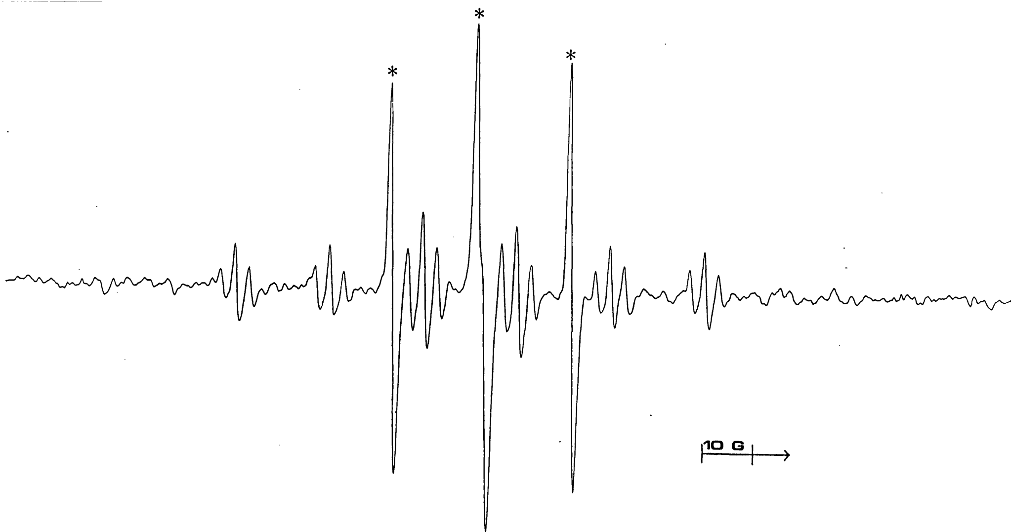
Figure 2.6 ESR spectrum of the mixture of radicals derived from a 1:2 molar mixture of cyclopentanone and t-butyl methyl ether in the absence of polarity reversal catalyst at 154 K. The lines marked with an asterisk arise from \text{Bu}^t\dot{\text{O}}\text{CH}_2 .
