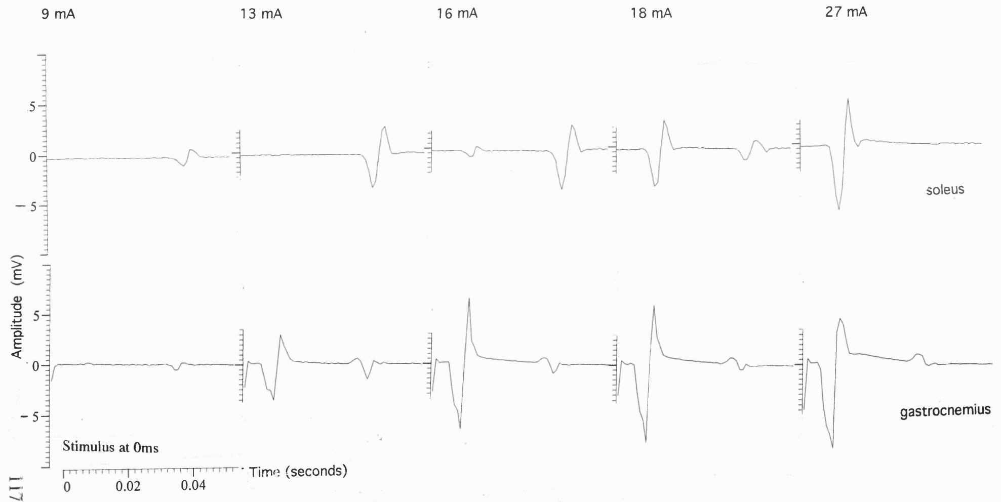
FIGURE 4.4 SIMULTANEOUS RECORDINGS FROM GASTROCNEMIUS AND SOLEUS AT DIFFERENT LEVELS OF INTENSITY OF STIMULATION
