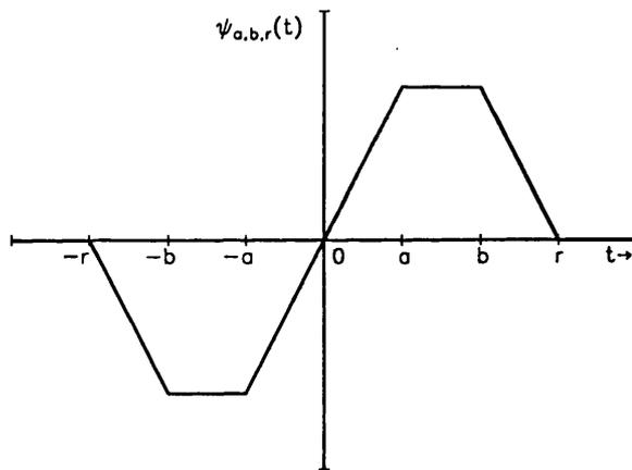
Figure 1.2: Shape of Hampel's three-part redescending  $\psi$ -function.
