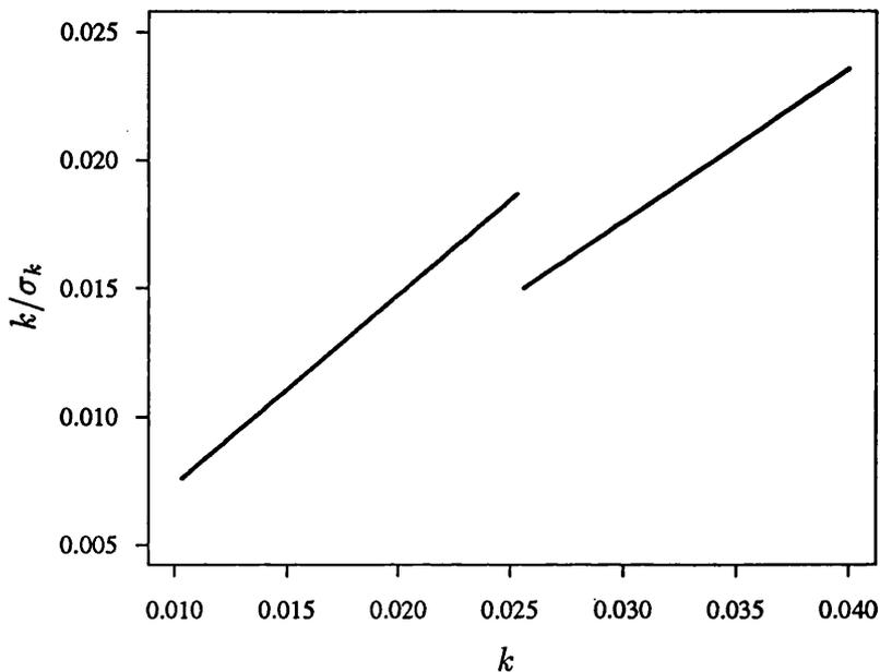
Figure 2.1: Discontinuity from use of Cauchy  $M$ -estimator on clustered data.
