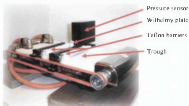
Figure 3.2. The Langmuir Blodgett trough was utilised in the experiments. The trough has two mechanical removable Teflon barriers. The pressure sensor was mounted on the edge of the trough and used a Wilhelmy plate to measure the surface pressure (reduction in surface tension). The volume of the trough was 0.50 cm x 13.5 cm and 8 cm. Tubing connectors was available for temperature control.
