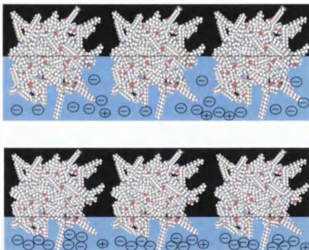
Figure 3.10. Examples of two possible arrangements of dendrimers at the air/water interface. The upper figure show a larger amount of dendrimer in the subphase (contact angle less than 90^\circ ) and the lower a smaller amount ( \theta > 90^\circ ). Depending on the arrangement of the dendrimer in the subphase, repulsion between them will increase, inter alia , the surface area per molecule increases.
