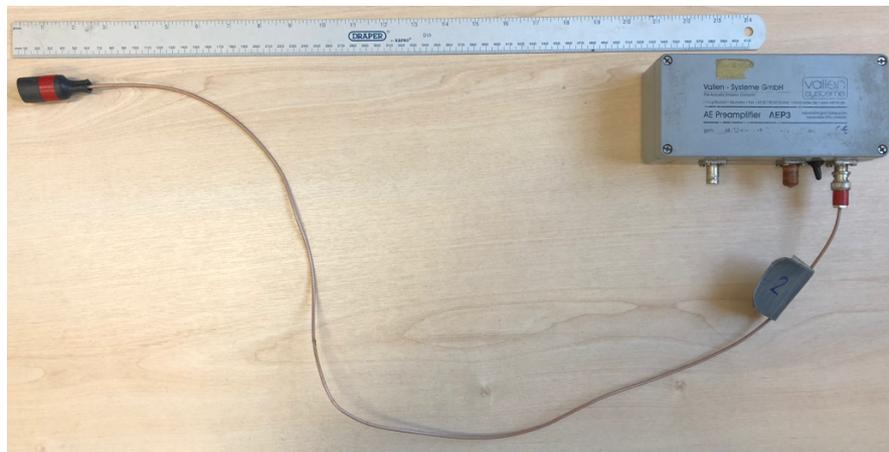
**Figure 2: Example of an AE transducer and Vallen pre-amplifier used in the friction tests**
