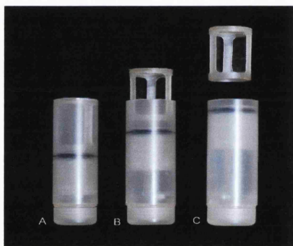
Figure 4.5 InteliSite ® companion device. A) Device sealed with cage inside the body, B) Cage partly expelled from body, C) Cage fully released and expelled from the body.
