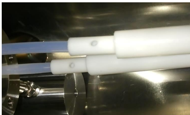
Figure 2.3: Image showing the pumping holes on the PTFE connectors. The size of the holes can be varied to change the amount of gas reaching the main chamber.
