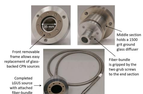
**Fig. 1.** Modular design of the LGUS source fabricated from aluminum. Clockwise: The CPN source element is securely held in a front plastic frame which is attached with screws to the middle section. The middle section holds a Thorlabs, Inc 1500 grit ground glass diffuser to both expand and homogenize the laser beam to a diameter of nearly 30 mm. The fiberbundle is gripped by the two grub screws on the end section which in turn is secured to the middle section with screws.
