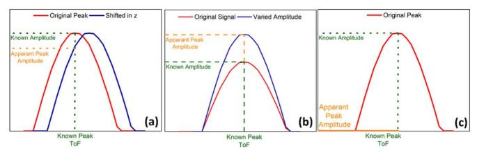
**Figure 1.** A number of potential peak variations in acoustic ToF analysis of Li-ion batteries including (a) a change in measured amplitude due to the interface physically moving in z, (b) a measured increase in the amplitude due to a change in the ratio of acoustic impedances at a given interface and (c) the complete absence of the interface being measured.
