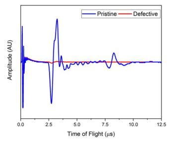
**Figure 6.** Ultrasonic ToF waveforms obtained in through transmission mode through the pristine and defective commercial cells shown in Fig. 5 showing large differences between the transmission signals due to the presence of the defect.
