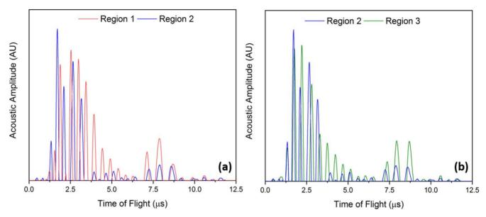
Figure 3. Example waveforms highlighting the relative change in displacement between the transducer and electrode layers caused by the ledge effect, showing a large variation throughout the waveforms between Region 1 and 2 and a similarity in waveforms until ca. 2  $\mu$ s between Region 2 and 3.
