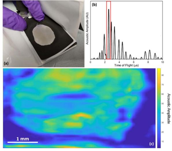
**Figure 4.** Diagnostic approach to identifying defects in cathode deposition (a) shown in a photograph prior to cell sealing (b) a single acoustic scan highlighting the ToF peak of interest at 2.5  $\mu$ s and (c) a 2D raster showing a region corresponding to that highlighted in the photograph demonstrating the efficacy of the technique.
