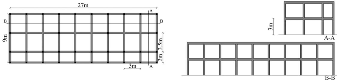
Figure 2: Geometry of the archetype building.
