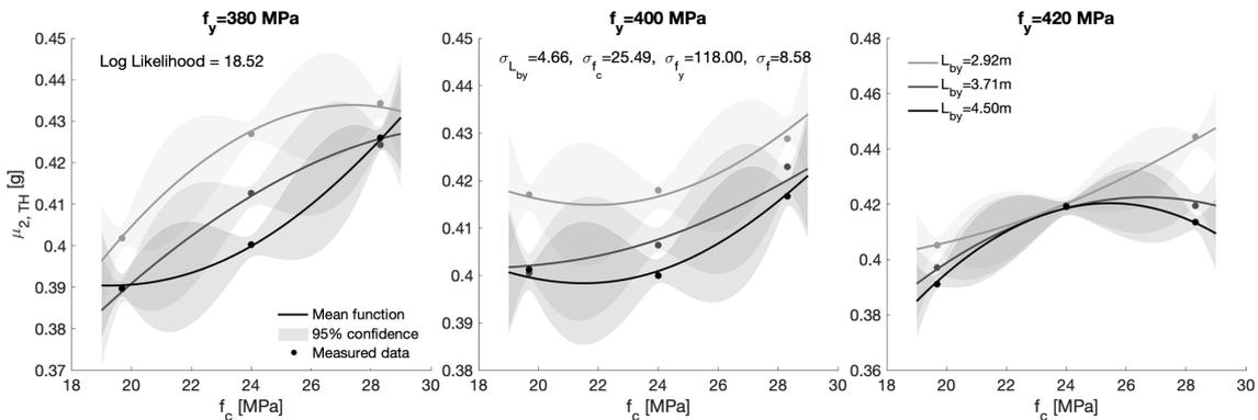
Figure 5: Pre-Code, transverse direction GP for the DS<sub>2</sub> fragility median based on full time-history.
