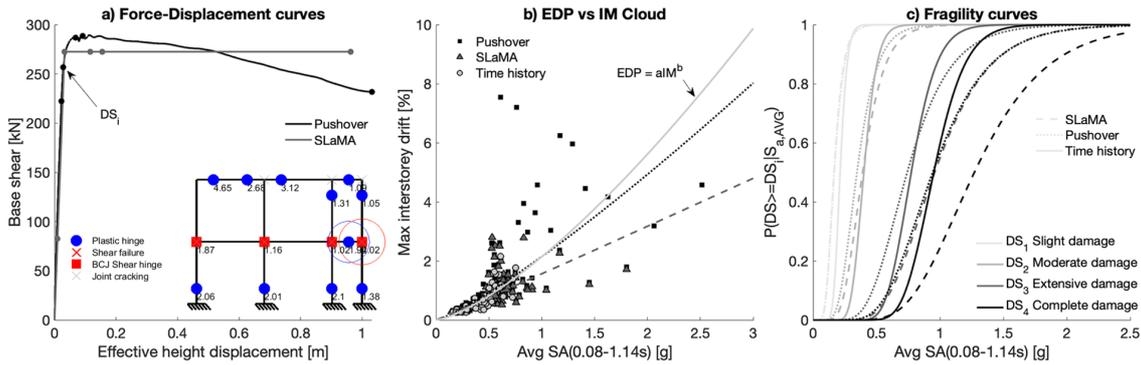
Figure 4: Transverse analysis results for the Pre-Code,  $L_{by}$ -4.5m,  $f_y$ -380MPa,  $f_c$ -24MPa building realisation.
