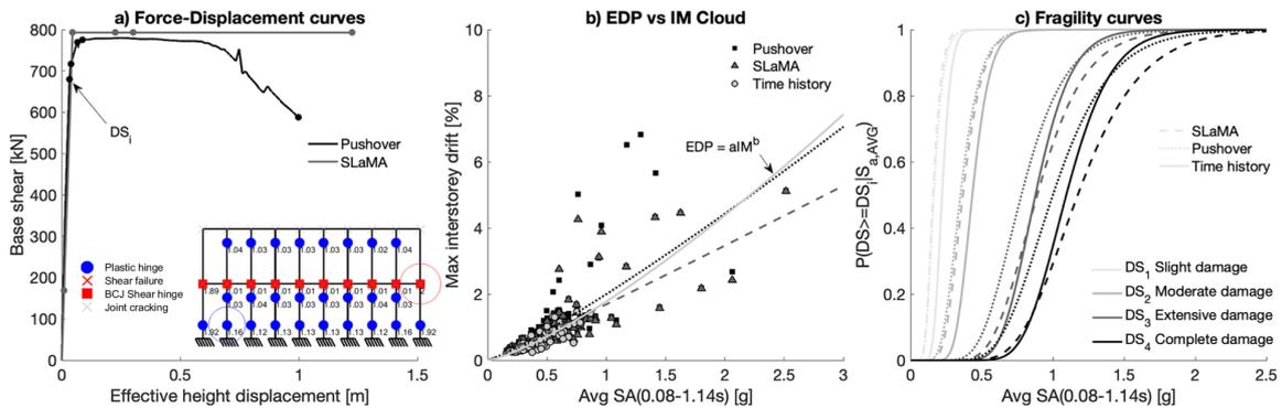
Figure 3: Longitudinal analysis results for the Low-Code, 9-bays,  $f_y$ -400MPa,  $f_c$ -19.7MPa building realisation.
