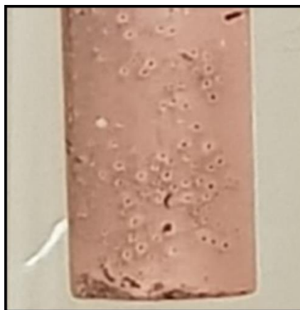
Figure 33: Image of the recovered Cu coating with noticeable holes probably created by H_2 gas evolution.
