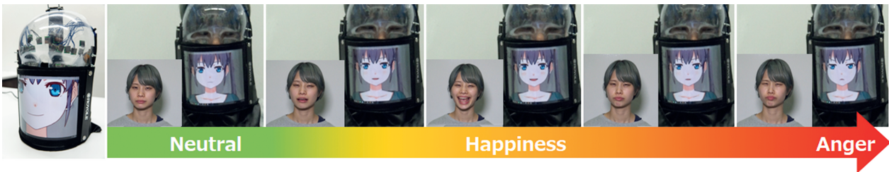
Figure 1: An oblique view image of a digital full-face mask display and the series of avatar animations reflecting the transition of the facial expression of the wearer
